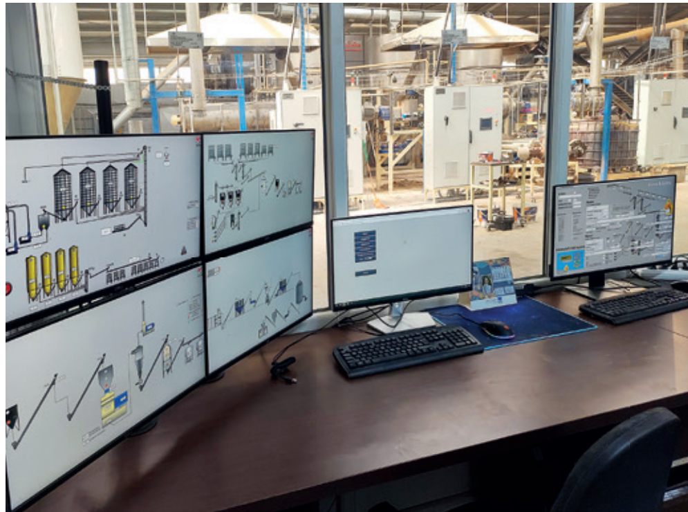
Control of a milling & mixing plant with HIMEL weighing computer
