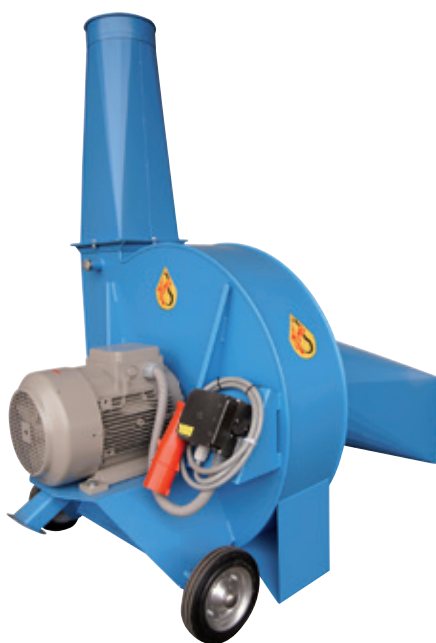
STM straw mill with electric motor
