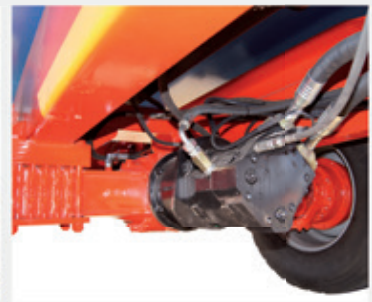
Axle drive with differential lock
