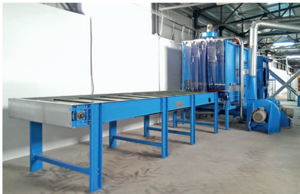
Stationary bale dissolver with feed table
