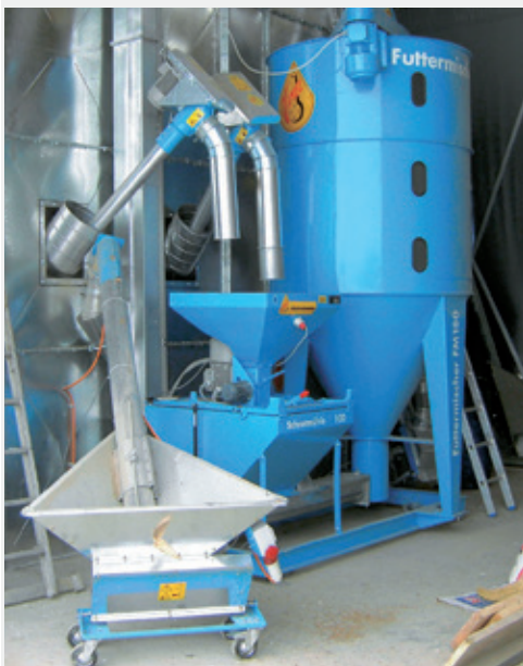
HIMEL grinding-mixing plant, feed mixer FMK 180 with SC mill
