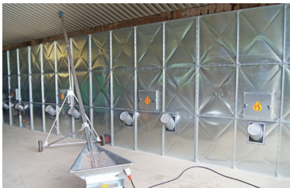
HIMEL rectangular silo with screw conveyor with hopper
